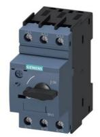
Circuit breaker size S0 for motor protection, CLASS 10 A-release 27...32 A N-release 400 A screw terminal Standard switching capacity
