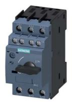
Circuit breaker size S0 for motor protection, CLASS 10 A-release 27...32 A N-release 400 A screw terminal Standard switching capacity with transverse auxiliary switches 1 NO+1 NC
