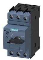
Circuit breaker size S0 for motor protection, CLASS 10 A-release 34...40 A N-release 480 A screw terminal Standard switching capacity
