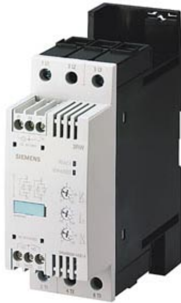
SIRIUS SOFT STARTER, SIZE S0, 12,5A, 7.5 KW / 400 V, AC 460...575 V, UC 24 V, SCREW CONNECTION
