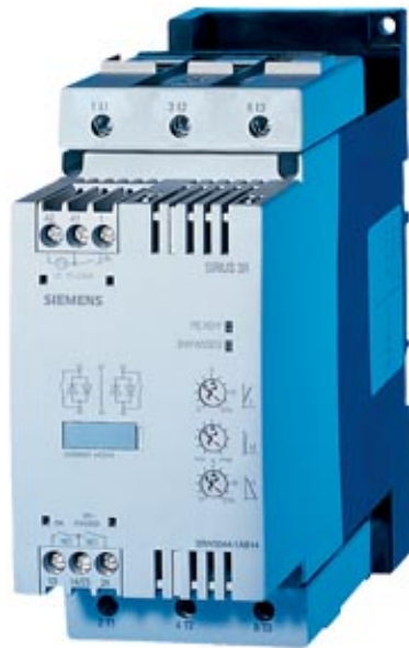
SIRIUS SOFT STARTER, SIZE S3, 75 A, 37 KW / 400 V, AC 200...460 V, UC 24 V, SCREW CONNECTION
