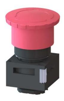
EMERGENCY STOP MUSHR. PUSHB., 22MM, ROUND, PLASTIC, RED, 40 MM, LATCHING, ROTATE TO UNLATCH; SHORT DESIGN, WITH HOLDER
