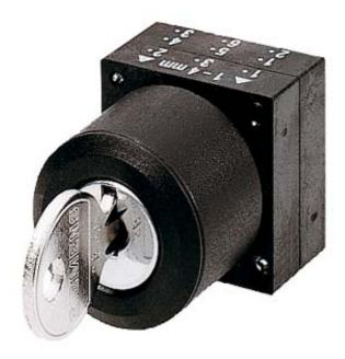
22MM PLASTIC ROUND ACTUATOR: RONIS LOCK WITH 2 KEYS 2 SWITCH POSITIONS O-I MAINTAINED CONTACT LOCK NUMBER SB 30, REMOVE O+I WITH HOLDER POSSIBLE SPECIAL LOCKS FOR RONIS KEYSWITCHES: SB31, 455, 421
