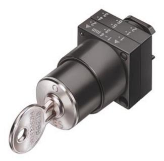
KEY-OPER. SWITCH CES, WITH KEY MONITORING, 22MM, ROUND, PLASTIC, LOCK NO SSG10, WITH 2 KEYS, 2 SWITCH POSITIONS O-I, LATCHING, ACTUATING ANGLE 50 DEG, 12/14 O'CLOCK REMOVAL POS. O, WITH HOLDER
