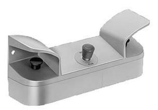
TWO-HAND OPERATOR PANEL FOR COMMAND DEVICES, 22MM, ROUND, ENCLOSURE MATERIAL PLASTIC, ENCLOSURE TOP PART GRAY, 3 COMMAND POSITIONS, 2 MUSHROOM PUSHBUTTONS, BLACK, 40MM, EACH WITH 1NO+1NC, 1 EMERGENCY-STOP MUSH. PUSHBUTTON, RED, 40MM, POSITIVE LATCHING, 2NC, WITH 8 PRESET BREAKING POINTS FOR FURTHER COMMAND DEVICES, WITH CABLE BREAK-THROUGHS FOR METRIC SCREW GLANDS
