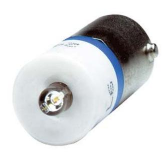
ACCESSORY / SPARE PART ROUND, 22MM/SQUARE, 26X26MM: LED SUPER-BRIGHT LAMPS, BASE BA 9S BULB DIAMETER 10MM RATED VOLTAGE 230V AC/DC OPERATIONAL CURRENT MAX. 15 MA GREEN
