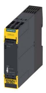
SIRIUS SAFETY RELAY OUTPUT EXTENSION 4RO WITH RELAY ENABLING CIRCUITS 4 NO CONTACTS + RELAY SIGNALING CIRCUIT 1 NC CONTACT US = 24 V DC SCREW CONNECTION
