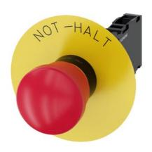
EMERGENCY STOP mushroom-type actuator, 22 mm, round, plastic, red, 40 mm, positive latching, according to EN ISO 13850, pull-to-unlatch mechanism, with yellow backing plate, inscription: NOT-HALT, with holder, 1 NO+1 NC, screw terminal
