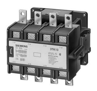
AC-1 CONTACTOR, 4-POLE, 200 A, MAIN CONTACTS 4 NO, AUXILIARY CONTACTS 2NO+2NC, AC OPERATION AC 220...230V 50HZ
