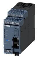
Basic unit SIMOCODE pro V PN GP , Ethernet/PROFINET IO, PN system redundancy, OPC UA server, Web server, transmission rate 100 Mbps, 1 x bus connection via RJ45, 4 I/3 Q freely parameterizable, Us: 24 V DC, input for thermistor connection Monostable relay outputs, expandable by 1 extension module(DM, TM, EM)
