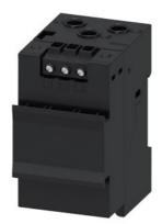
Current/voltage measuring module V2; Set current 3...40 A, Voltage measurement up to 690 V, Overall width 45 mm, Straight-through transformer, basic unit required pro V PB, pro V MR, pro V PN or pro V EIP
