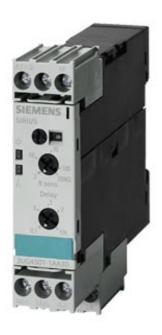
ANALOG MONITORING RELAY FILL LEVEL MONITORING RESISTANCE MONITORING FROM 2 TO 200 KOHM OVERSHOOT AND UNDERSHOOT AC/DC 24 TO 240V DC AND AC 50 TO 60 HZ 2-POINT OR 1-POINT CONTROL TRIPPING DELAYED 0.5 TO 10S 1 CHANGEOVER CONTACT SCREW TERMINAL REPLACEMENT PRODUCT F. 3UG3501
