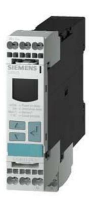
Digital monitoring relay Voltage monitoring, 22.5 mm from 17-275 V AC/DC 0vershoot and undershoot selfsupplied 50 to 60 Hz DC and AC Noise pulses delay 0.1 to 20 s Hysteresis 0.1 to 150 V 1 change-over contact with or without fault buffer screw terminal Successor product for 3UG3534, 3UG3535
