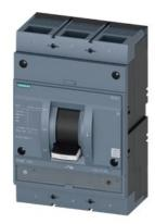
circuit breaker 3VA1 IEC frame 1000 breaking capacity class M Icu=55kA @ 415V 3-pole, line protection TM240, ATAM, In=800A overload protection Ir=560A...800A short-circuit protection Ii=5...10 x In nut keeper kit
