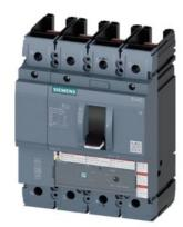
circuit breaker 3VA5 UL frame 250 breaking capacity class H 65kA @ 480 V 4-pole, line protection TM240, ATAM, In=175A without overload protection Ir=140A ...175A short circuit protection Ii=5...10 x In neutral protection 1 w/o connection
