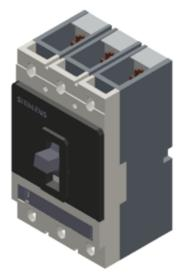
CIRCUIT-BREAKER VL 160N STANDARD BREAKING CAPACITY ICU=55KA / 415 V AC 3 POLE, LINE PROTECTION OVERCURRENT RELEASE TM, LI IN=125A, RATED CURRENT IR=100-125A, OVERLOAD II=625-1250A, SHORT CIRCUIT WITH SCREW CONNECTION
