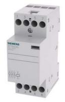
INSTA contactor with 4 NO contacts Contact for 230 V AC, 400V 25A Control AC/24 V DC
