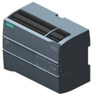
SIPLUS S7-1200 CPU 1215C DC/DC/DC based on 6ES7215-1AG40-0XB0 with conformal coating, -20...+60 °C, compact CPU, DC/DC/DC, 2 PROFINET ports, onboard I/O: 14 DI 24 V DC 10 DQ 24 V DC 0.5 A 2 AI 0-10 V DC, 2 AQ 0-20 mA DC, power supply: DC 20.4-28.8 V DC, program/data memory 125 KB
