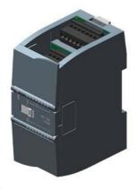
SIPLUS S7-1200 SM 1234 4AI/2AQ based on 6ES7234-4HE32-0XB0 with conformal coating, -20...+60 °C, analog I/O +/-10 V: 14-bit resolution or 0-20 mA: 13-bit resolution
