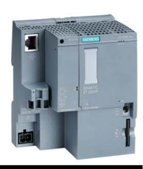
SIPLUS ET 200SP CPU 1510SP-1 PN -40...+60 °C STARTUP TEMP.: -25 °C WWITH CONFORMAL COATING BASEDON 6ES7510-1DJ01-0AB0 . CPU 1510SP-1 PN FOR ET 200SP, CENTRAL PROCESSING UNIT WITH WORKING MEMORY 100 KB FOR PROGRAM AND 750 KB FOR DATA, 1. INTERFACE: PROFINET IRT WITH 3 PORT SWITCH, 72 NS BIT-PERFORMANCE, SIMATIC MEMORY CARD NECESSARY, BUSADAPTER NECESSARY FOR PORT 1 AND 2
