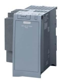
SIPLUS S7-1500 CPU 1516-3 PN/DP TX RAIL -40 ... +70°C TX with 85°C for 10 min with conformal coating based on 6ES7516-3AN01-0AB0 . CPU without display with 1 MB RAM for program and 5MB for data, 1st interface: PROFINET IRT with 2-port switch, 2nd interface: Ethernet, 3rd interface: PROFIBUS, 10 ns bit performance, SIMATIC Memory Card required
