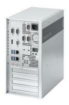
SIMATIC IPC527G (Box PC); Core i5-6500 (4C/4T, 3.2 (3.6) GHz); 256 GB SSD, internal; 8 GB DDR4; Windows 7 Ultimate 64 bit, MUI; 2x Gigabit Ethernet (IE/PN); 1x display port, 1x VGA; 4x USB 3.0, 2x USB 2.0; 2x RS232/485/422 (can be selected); 2x RS232, 1x 8bit DIO, 2x PCI; 1x PCIe x16, 1x PCIe x1; 100/240 V AC power supply without line cable
