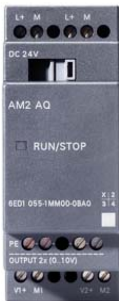
LOGO! AM2 AQ EXPAN. MODULE, PU: DC 24V, 2AQ, 0-10V
