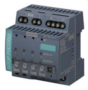
SITOP PSE200U SELECTIVITY MODULE 3A SITOP PSE200U 3 A 4-channel selectivity module input: 24 V DC/12 A output: 24 V DC/4x 3 A threshold adjustable 0.5-3 A with status message per output
