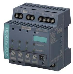
SITOP PSE200U SELECTIVITY MODULE 10A SITOP PSE200U 10 A 4-channel selectivity module input: 24 V DC/40 A output: 24 V DC/4x 10 A threshold adjustable 3-10 A with status message per output
