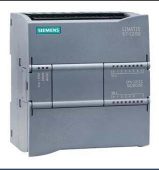
SIMATIC S7-1200, CPU 1212C, COMPACT CPU, DC/DC/DC, ONBOARD I/O: 8 DI 24V DC; 6 DO 24 V DC; 2 AI 0 - 10V DC, POWER SUPPLY: DC 20.4 - 28.8 V DC, PROGRAM/DATA MEMORY: 25 KB
