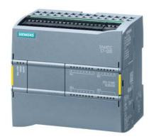
SIMATIC S7-1200F, CPU 1214 FC, compact CPU, DC/DC/DC, onboard I/O: 14 DI 24 V DC; 10 DO 24 V DC; 2 AI 0-10 V DC, power supply: DC 20.4-28.8 V DC, program/data memory 200 KB
