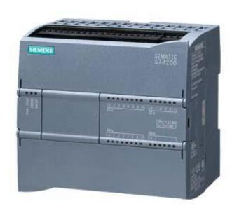
SIMATIC S7-1200, CPU 1214C, COMPACT CPU, DC/DC/RELAY, ONBOARD I/O: 14 DI 24V DC; 10 DO RELAY 2A; 2 AI 0 - 10V DC, POWER SUPPLY: AC 20 4 - 28 8 V D
