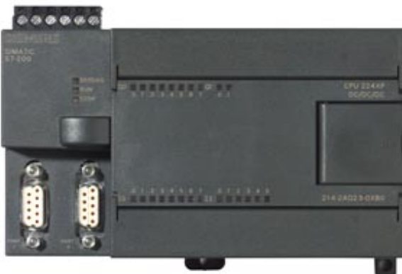
SIMATIC S7-200, CPU 224XP COMPACT UNIT, DC POWER SUPPLY 14 DI DC/10 DO DC, 2 AI, 1 AO 12/16 KB CODE/10 KB DATA, 2 PPI/FREEPORT PORTS
