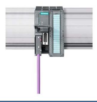
SIMATIC S7-300, CPU 313C-2 PTP COMPACT CPU WITH MPI, 16 DI/16 DO, 3 FAST COUNTERS (30 KHZ), INTEGRATED INTERFACE RS485, INTEGRATED 24V DC POWER SUPPLY, 128 KBYTE WORKING MEMORY, FRONT CONNECTOR (1 X 40PIN) AND MICRO MEMORY CARD REQUIRED
