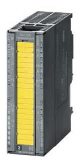
SIMATIC S7, DIGITAL OUTPUT SM326, F-DO10 X DC24V/2A PP, FAILSAFE DIGITAL OUTPUTS FOR SIMATIC S7F SYSTEMS WITH DIAGNOST. INTERRUPT, LVV, UP TO CATEGORY 4 (EN954-1)/ SIL3 (IEC61508)/PLE (ISO13849), 1 X 40 PIN
