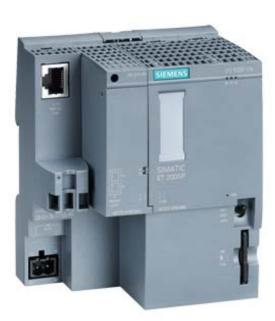
SIMATIC DP, CPU 1512SP-1 PN FOR ET 200SP, CENTRAL PROCESSING UNIT WITH WORKING MEMORY 200 KB FOR PROGRAM AND 1 MB FOR DATA, 1. INTERFACE: PROFINET IRT WITH 3 PORT SWITCH, 48 NS BIT-PERFORMANCE, SIMATIC MEMORY CARD NECESSARY, BUSADAPTER NECESSARY FOR PORT 1 AND 2
