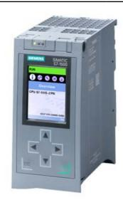
SIMATIC S7-1500, CPU 1515-2 PN, CENTRAL PROCESSING UNIT WITH WORKING MEMORY 500 KB FOR PROGRAM AND 3 MB FOR DATA, 1. INTERFACE, PROFINET IRT WITH 2 PORT SWITCH, 2. INTERFACE, ETHERNET, 30 NS BIT-PERFORMANCE, SIMATIC MEMORY CARD NECESSARY
