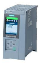
SIMATIC S7-1500, CPU 1515-2 PN, central processing unit with work memory 1 MB for program and 4.5 MB for data, 1st interface: PROFINET IRT with 2-port switch, 2nd interface: PROFINET RT, 6 ns bit performance, SIMATIC Memory Card required \*\*\* approvals and certificates according to entry 109817466 at support.industry.siemens.com to be considered! \*\*\*
