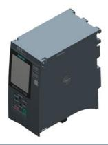
SIMATIC S7-1500F, CPU 1515F-2 PN, central processing unit with 1.5 MB work memory for program and 4.5 MB for data, 1st interface: PROFINET IRT with 2-port switch, 2nd interface: PROFINET RT, 6 ns bit performance, SIMATIC Memory Card required \*\*\* approvals and certificates according to entry 109817466 at to be considered! \*\*\*
