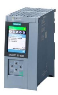
SIMATIC S7-1500F, CPU 1516F-3 PN/DP, central processing unit with 1.5 MB work memory for program and 5 MB for data, 1st interface: PROFINET IRT with 2-port switch, 2nd interface: PROFINET RT, 3rd interface: PROFIBUS, 10 ns bit performance, SIMATIC Memory Card required
