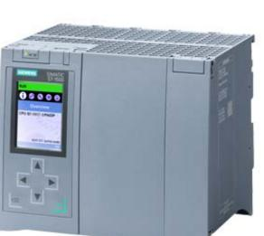
SIMATIC S7-1500, CPU 1517-3 PN/DP, CENTRAL PROCESSING UNIT WITH WORKING MEMORY 2 MB FOR PROGRAM AND 8 MB FOR DATA, 1. INTERFACE: PROFINET IRT WITH 2 PORT SWITCH, 2. INTERFACE: PROFINET RT, 3. INTERFACE: PROFIBUS, 2 NS BIT-PERFORMANCE, SIMATIC MEMORY CARD NECESSARY
