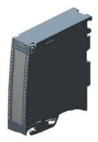
SIMATIC S7-1500, digital output module DQ 32x24 V DC/0.5A HF; 32 channels in groups of 8; 4 A per group; single-channel diagnostics; substitute value: the module supports the safety-oriented shutdown of load groups up to SILCL2 acc. to EN 62061:2005 + A2:2015, and Category 3 / PL d according to EN ISO 13849-1:2015. front connector (screw terminals or push-in) to be ordered separately
