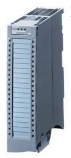
SIMATIC S7-1500 Analog output module AQ8xU/I HS, 16 bit resolution, accuracy 0.3%, 8 channels in groups of 8; Diagnostics; Substitute value 8 channels in 0.125 ms Oversampling; Delivery including infeed element, shield bracket and shield terminal: Front connector (screw terminals or push-in) to be ordered separately
