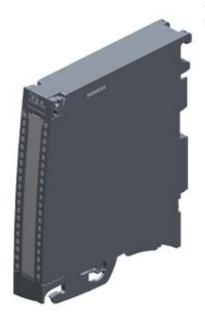
SIMATIC S7-1500, Analog output module AQ 2x U/I ST, 16 bit resolution, Accuracy 0.3%. 2 channels in groups of 2, diagnostics; Substitute value incl. push-in front connector, infeed element, shield bracket, shield terminal
