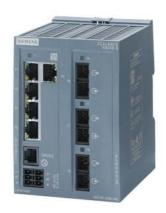
SCALANCE XB205-3 managed Layer 2 IE Switch 5x IEC 62443-4-2 certified; 10/100 Mbit/s RJ45 ports 3x MM FO SC-port 1x console port, diagnostics LED redundant power supply; IEC 62443-4-2 certified; temperature range 0 °C to +60 °C; DIN-rail mounting; default EtherNet/IP.
