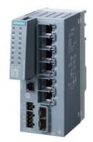
SCALANCE XC206-2SFP G manageable Layer 2 IE switch; IEC 62443-4-2 certified; 6x 10/100/1000 Mbit/s RJ45 ports; 2x 1000 Mbit/s SFP; 1x console port; diagnostics LED; redundant power supply; temperature range -40 °C to +70 °C; assembly: DIN rail/S7 mounting rail/wall; redundancy functions; office features (RSTP, VLAN,...); PROFINET IO device; Ethernet/IP-compliant; C-PLUG slot;
