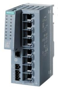
SCALANCE XC208 manageable layer 2 IE Switch; 8x 10/100 Mbit/s RJ45 ports; 1x console port; Diagnostic LED; Redundant power supply; Temp. range -40°C to +70 °C Mounting: Standard Mounting Rail/S7 Profile Rail/Wall Office redundancy functions features (RSTP, VLAN ,...); PROFINET IO device Ethernet/IP-compliant C-PLUG shaft;
