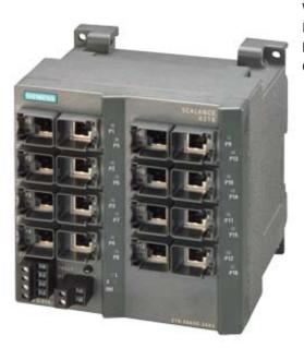
SCALANCE X216, MANAGED IE SWITCH, 16 X 10/100MBIT/S RJ45 PORTS, LED DIAGNOSTICS, FAULT SIGNAL. CONTACT WITH SET BUTTON REDUNDANT POWER SUPPLY, PROFINET-IO DEVICE, NETWORK- MANAGEMENT, INTEGRATED REDUNDANCY MANAGER, INCL. ELECTRONIC MANUAL ON CD, C-PLUG OPTIONAL
