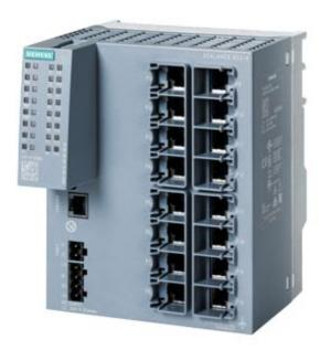
SCALANCE XC216 manageable layer 2 IE Switch; 16X 10/100 Mbit/s RJ45-Ports; 1x console port, Diagnostic LED; Redundant power supply; Temp. range -40°C to +70 °C Mounting: Standard Mounting Rail/S7 Profile Rail/Wall Office redundancy functions features (RSTP, VLAN ,...); PROFINET IO Device; Ethernet/IP compliance C-PLUG shaft;
