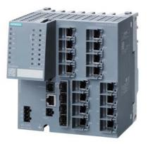
SCALANCE XM416-4C; managed modular IE switch; 16x 10/100/1000 Mbit/s RJ45; 4x 100/1000 Mbit/s SFP; contains 4 combo ports; in total 16 ports can be used; expandable to 24 ports electrical or optical; assembly: DIN rail/S7 mounting rail, PROFINET IO device; redundancy functions; office features (RSTP, VLAN, IGMP,...); C-plug in scope of delivery; Layer 3 with key plug available
